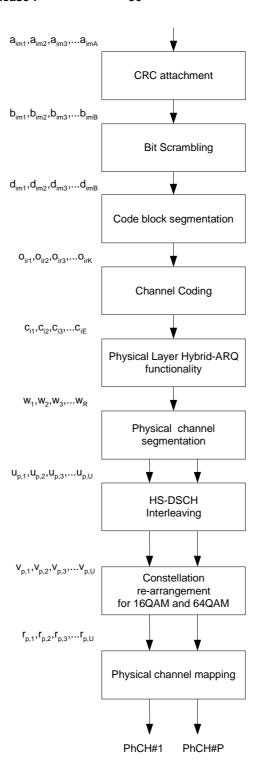
Figure 16: Coding chain for HS-DSCH
